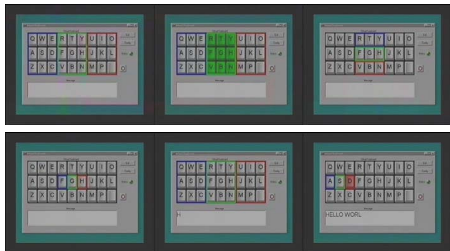
Figure 12: Example of virtual keyboard. The figure shows a sequence of frames during the writing of a message (from left to right and top down). At the beginning, top left panel, the keyboard is divided in three parts, each associated to one of the mental tasks and using the same colors as during the training. Once the neural classifier recognizes the same mental task three times in a row, the corresponding part of the keyboard is selected (top center panel). In this case is the green area, which remains shadowed for 3.5 seconds to give the user the possibility to undo the selection in case it is wrong. Then, this part is divided again in three (top right panel). After a block of this second level is selected, it is still split in three to yield the choice among three letters (bottom left panel). The user then selects the letter with the red color (h) that is written into the message part and the whole process starts over again (bottom center panel). The bottom right panel shows the selection of the last letter in the message (reproduced from (Millán, 2003))
