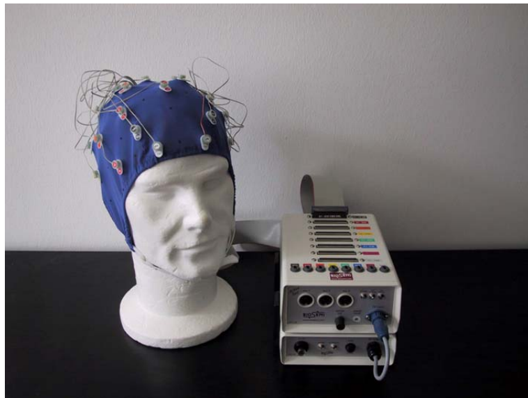
Figure 9: Portable EEG system used at the IDIAP Research Institute. It is a commercial BioSemi ActiveTwo system
